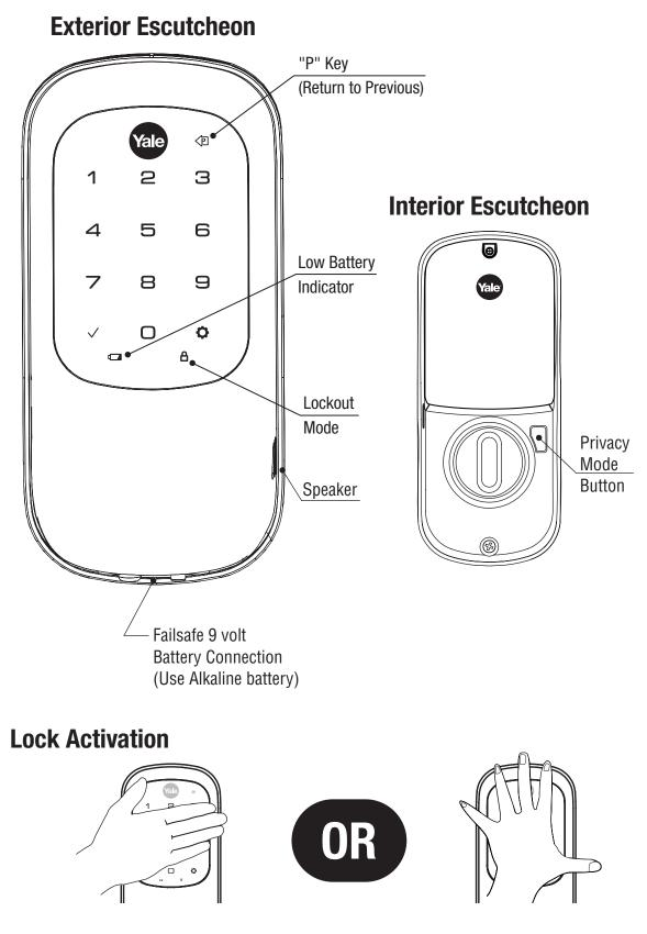
Master PIN Code must be created before any further programming. Max User Codes = 250 with Network Module. Max User Codes = 25 without.
