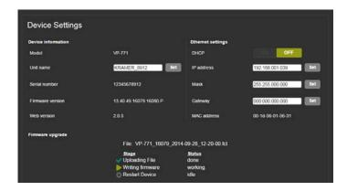
Figure 66: The Device Settings Page - Writing the Firmware
