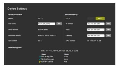
Figure 67: The Device Settings Page - Firmware Upgrade Waiting for Restart
