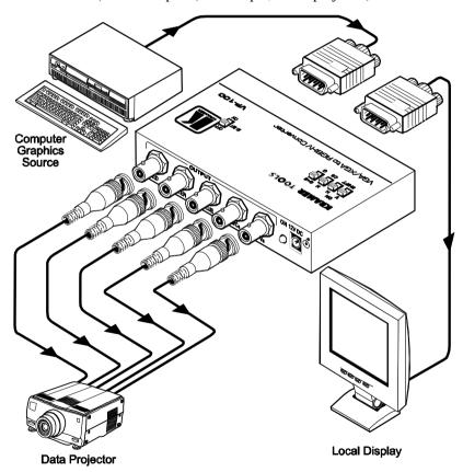
Figure 2: VP-100 VGA/XGA to RGBHV Converter Connections
