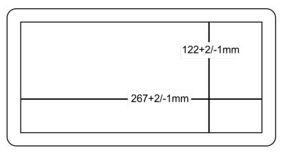
Figure 5: Cut out Dimensions
