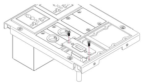
Figure 5: Mount the Inserts (After Installing the Kit)
