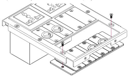
Figure 2: T-4INSERT Installation, Step 1
