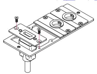
Figure 4: Mount the Inserts (Before Installing the Kit)
