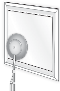
Option 1: Apply the booster directly to the window (ideally, at a window corner) using the provided adhesive.
