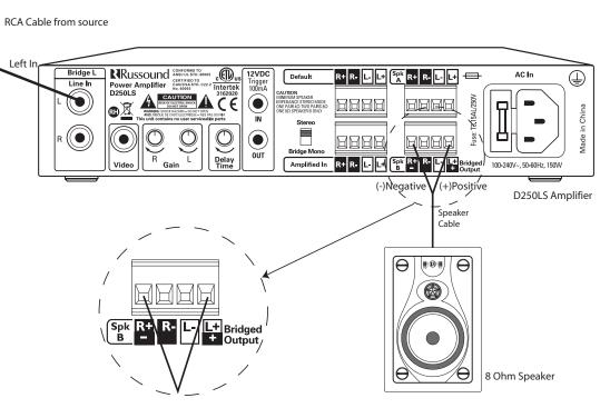
Connections for bridged mode operation
