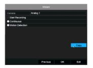
Once you have made the choices for the selected camera, you have two options for how to continue. You can either select a new camera using the dropdown menu at the top of the dialog box and make choices for it manually, or else you can press the **Copy** button.
