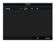
When you press **Copy**, a new dialog box opens. You can copy the current camera's settings to any or all of the other cameras in the system. Selecting the **Analog/Digital** button at the left automatically selects all analog or digital cameras on the system. You can also select or deselect the cameras individually by clicking their boxes.
