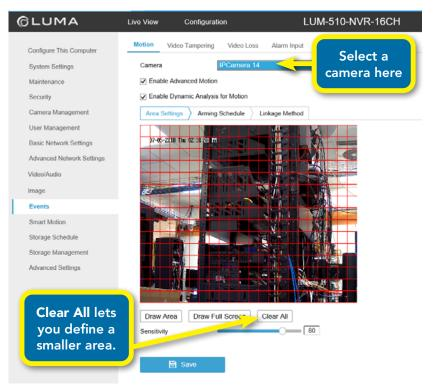
Select a camera in the dropdown at the top, and ensure motion detection is enabled with the checkbox.
