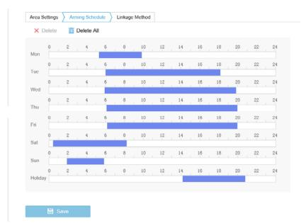
Be sure to fill the entire 24-hour period so that there are no lapses; schedules are inactive unless assigned. Schedule gaps smaller than ten minutes may be hard to see, especially if they occur at the top of the hour.
