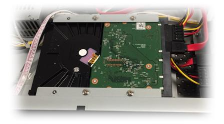
Remove the four screws that hold the hard drive in place and carefully slide the hard drive out.
