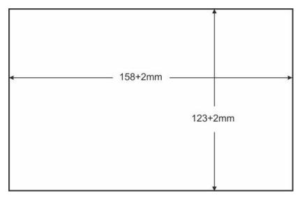
Figure 3: Cut-out Dimensions (not to scale)
