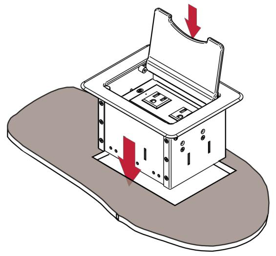
Figure 4: Inserting TBUS-3US-22 into the Table Opening
