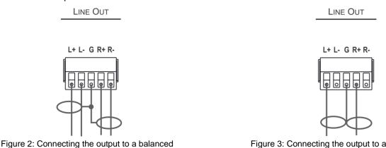
Figure 3: Connecting the output to an unbalanced stereo audio acceptor
