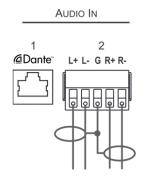
Figure 4: Connecting a balanced stereo audio source to the balanced input
