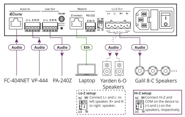
Figure 1: Connecting to the PA-240Net Rear Panel
