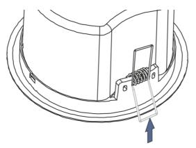
Figure 6: Pushing the Spring Clamps
