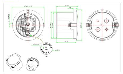
Figure 11: Galil 2-C Mechanical Drawing
