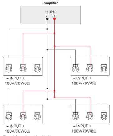
Figure 9: Square Layout Parallel Wiring
