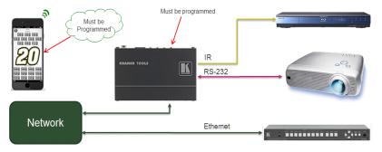
Figure 1: FC-26 Controlling Devices Remotely Using K-Touch 3.0 over a LAN
