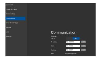
**Note**: The FC-26 is dispatched from the factory with the DHCP enabled and a random IP address. This means that if the device is connected to a LAN, you must identify the IP address of the FC-26 in order to connect to it. This can be done by using K-LAN Configurator to discover the IP address of the FC-26. This is available for download from our website at http://www.kramerav.com.
