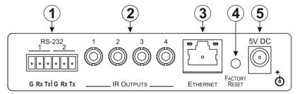
Figure 3: FC-26 Ethernet Controller Rear Panel
