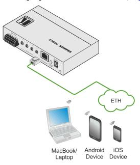
Figure 4: Connecting the FC-26 for Initial Configuration
