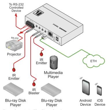
Figure 6: Connecting the FC-26 Ethernet Controller
