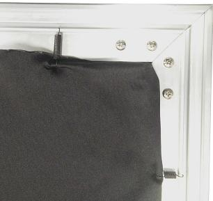
3. <u>Secure the remainder of the black backing.</u> The black backing should now be secured at the corners, but will be loose along the edges. At the center and several other mounting points along each edge, release the springs from the screen tension rods and lay the black backing over the rod, then reattach the springs. This will effectively tuck the black backing between the tension rod and each spring so that it will be secured in place. Your black backing is now properly installed.
