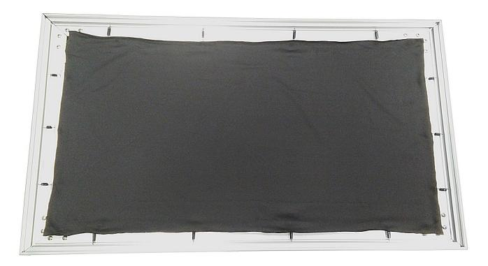
2. <u>Secure the black backing at each corner.</u> Release the two springs closest to each corner from the tension rods. Lay the black backing over the rod and hook the springs back over the tension rod and the black backing. Tuck the very corner of the material behind the tension rods to hold it firmly in place.
