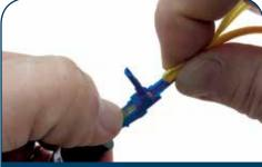
7. Slide activator tab towards connector tip. Remove from VFL. Ensure fiber is straight, hold Kevlar to one side, close hinge, install dust cap.
