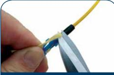
8. Slide boot forward and thread one full turn to "lock in" Kevlar strands. Cut Kevlar close to boot. Tighten boot until secure.
