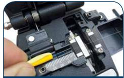
5. Cleave fiber measuring from cable jacket. For SSF<sup>™</sup> LC = 24mm.<sup>2</sup>
