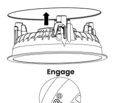
4. Place the mount in the hole and press the three buttons to engage the dog ears.
