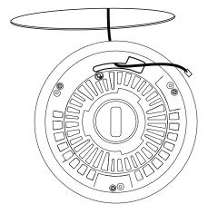
Pull the category cable through the mount's cable management hole. If the mount must be tied off, use the safety strap bar at the top of the mount.
