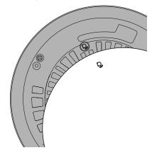
Connect the category cable to the AP, then align the Araknis logo under the mount's cable management hole and the logo on the AP to help you guide the AP into place.
