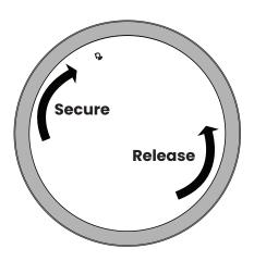
7. Gently push the AP and turn it clockwise to lock it into place. To release the AP, gently push and turn it counter-clockwise.
