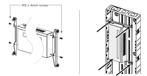
NOTE: The switch can only be mounted to the structured wiring can with the Ethernet ports facing right or left.
