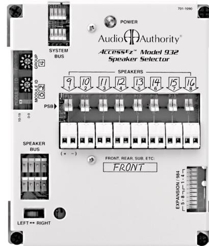
**Figure 26.** A Model 932 Speaker Selector, set to Group 4, Module 2, (Front Speaker Group, products 9-16). This is the LEFT module.
