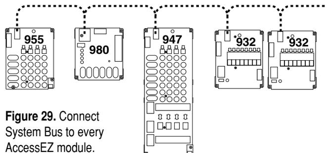
**Figure 29.** Connect System Bus to every AccessEZ module.
