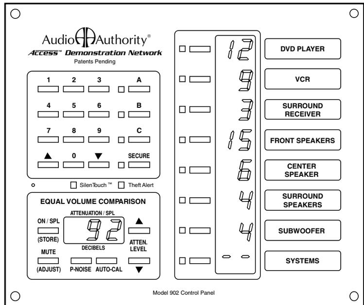
**Figure 21.** This is how Product Groups appear on the 902 Control Panel. The display shows which product in each group is selected.
