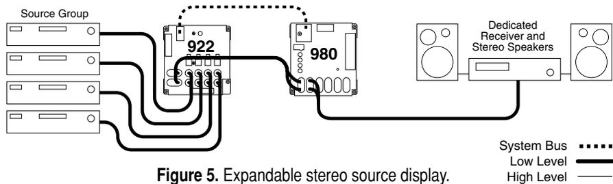
Figure 5. Expandable stereo source display.
