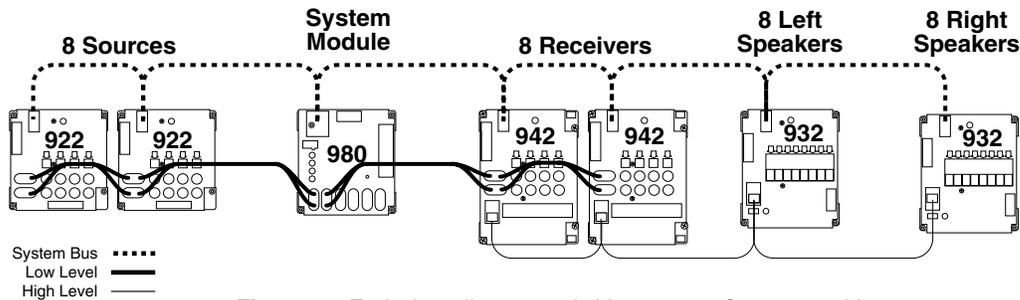
**Figure 11.** Typical small stereo switching system. Sources could include CD Players and/or playback-only Tape Decks.
