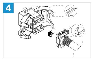
Check that the wired cap is aligned properly. Insert it into the keystopne and close the clamps.
