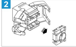
Open the clamps and remove the cap.
