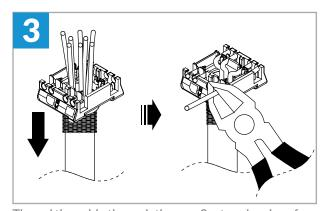
Thread the cable through the cap. Seat each color of wire into its matching cap position. Trim excess wire.
