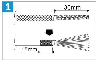
Remove 30mm of the cable jacket. Untwist and straighten the wires. Keep 15mm of the braid foil.
