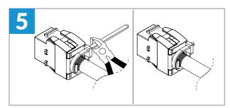
Wrap the supplied cable tie around the wired cap as shown, then tighten it. Trim the cable tie.
