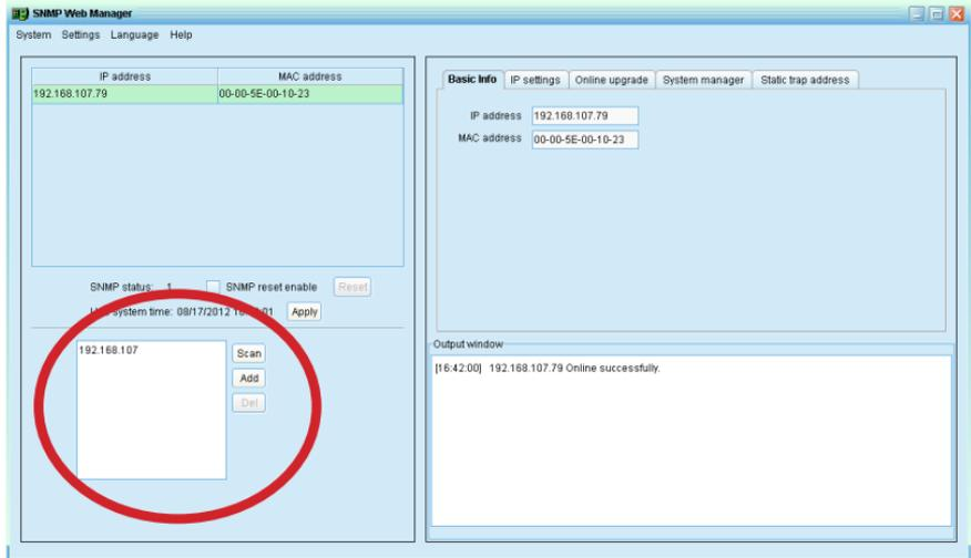
In the search box (circled) you can enter a partial or complete IP address to search for matching devices in the network. By default, the SNMP web manager has the IP address 192.168.102.230, with a subnet mask 255.255.255.0 and gateway 192.168.102.1.
