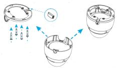
7. Secure the screws, lock the sphere section, and complete the installation.
