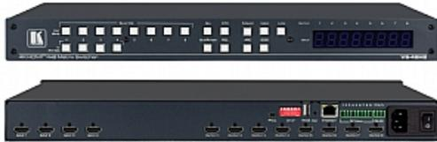
VS-48H2 is a high-performance 4x8 matrix switcher for 4K@60Hz (4:4:4) HDR signals and digital audio routing. It reclocks and equalizes the signals and can route any one of 4 HDMI, HDCP-compliant sources (selectable) to any or all outputs simultaneously. VS-48H2 offers unmatched audio flexibility where any embedded digital audio input can be routed to any digital output in addition to eight ARC sources to produce an equivalent 12x12 audio matrix
