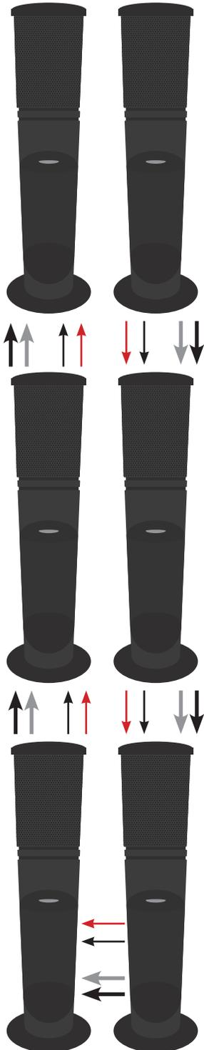
Parallel each LS. 32 in a "daisy chain" configuration for both speaker wiring and DC lighting.
