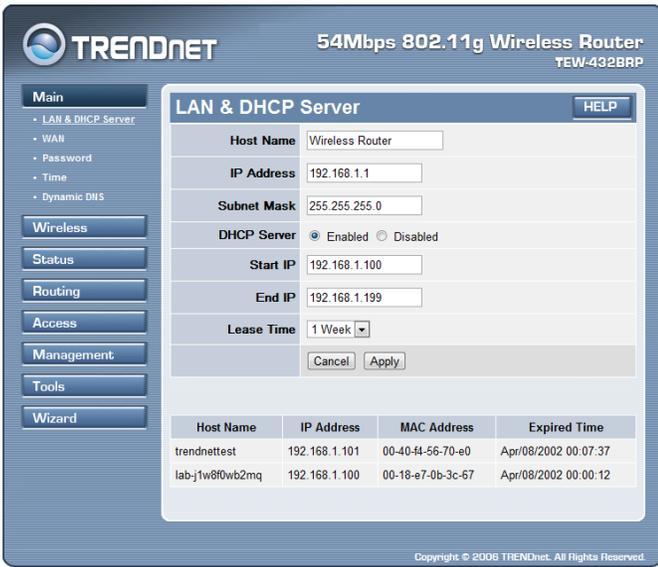
The screenshot shows the Trendnet web interface for a 54Mbps 802.11g Wireless Router (TEW-432BRP). The 'LAN & DHCP Server' configuration page is displayed. The DHCP Server is enabled, and the configuration includes a host name, IP address, subnet mask, start and end IP addresses, and a lease time of 1 week. A table below the configuration shows the DHCP server's current state for two clients.
