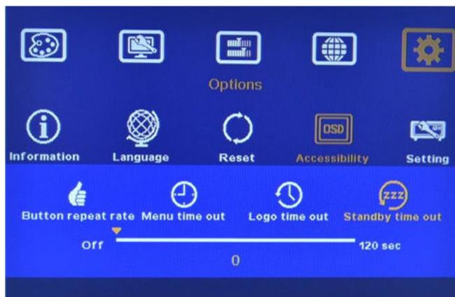
The default setting for [Standby Time Out] is 60 seconds. MLT-PROWALL-4K will automatically cut off output signal if no input signal is detected after 60 seconds. The time can be set by user. If the time is set to "0", then MLT-PROWALL-4K will not turn off the output signal even no input signal is detected.
