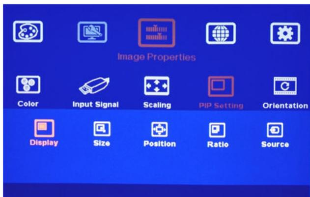
If user wants to keep PIP setting while system power on, user needs to set all [Main Input] Dip SW at OFF position and select input signal by OSD menu.
