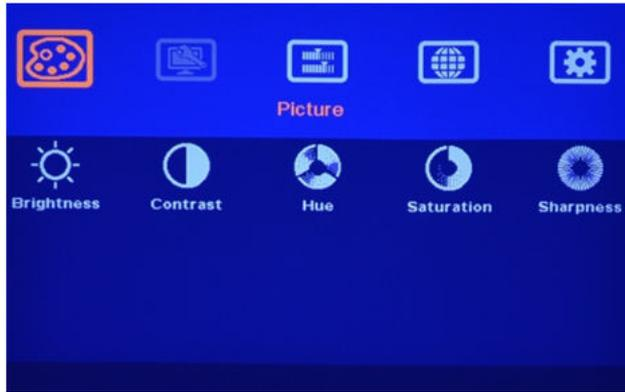
[Picture] menu is to adjust the color properties for the entire display unit (4x LCD). It can't do individual colour adjustment for each LCD. When the input signal is in YUV domain, all the items under menu are free to be accessed. If the input signal is in RGB domain, only [Brightness] and [Contrast] can be adjusted. User can do further separate RGB individual color adjustment under [Image Properties] menu.
