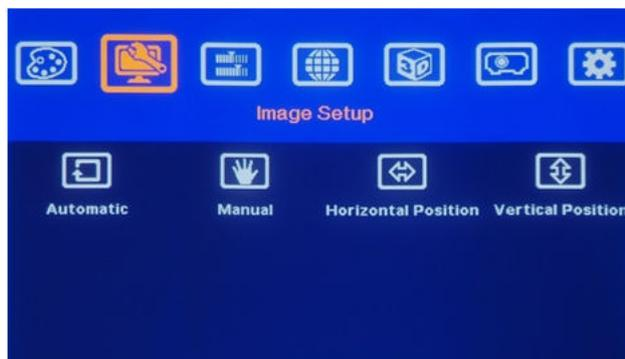
[Image Setup] menu can only be activated when video input is from DVI-I input port with analog VGA input signal.
