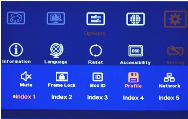
Five indexes can be chosen to save MLT-PROWALL-4K settings and can be recalled by IR remote controller or RS232 via [Load] menu under [Profile]
