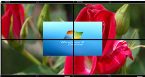
POP: to select POP (Picture outside Picture) display mode. User can select maintain original image aspect ratio or full screen mode through [Scaling] OSD menu under [Image properties]. If user set the system through Dip SW, user can select [POP Raw] and [POP Full] directly from front panel.
