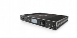
KDS-SW3-EN7 is an auto switcher and advanced encoder for streaming a selected video signal at 4K via Ethernet over copper cable in unicast (one-to-one) or multicast (one-to-many) configurations. It can add digital audio Dante, USB, IR, RS-232, or CEC signals
