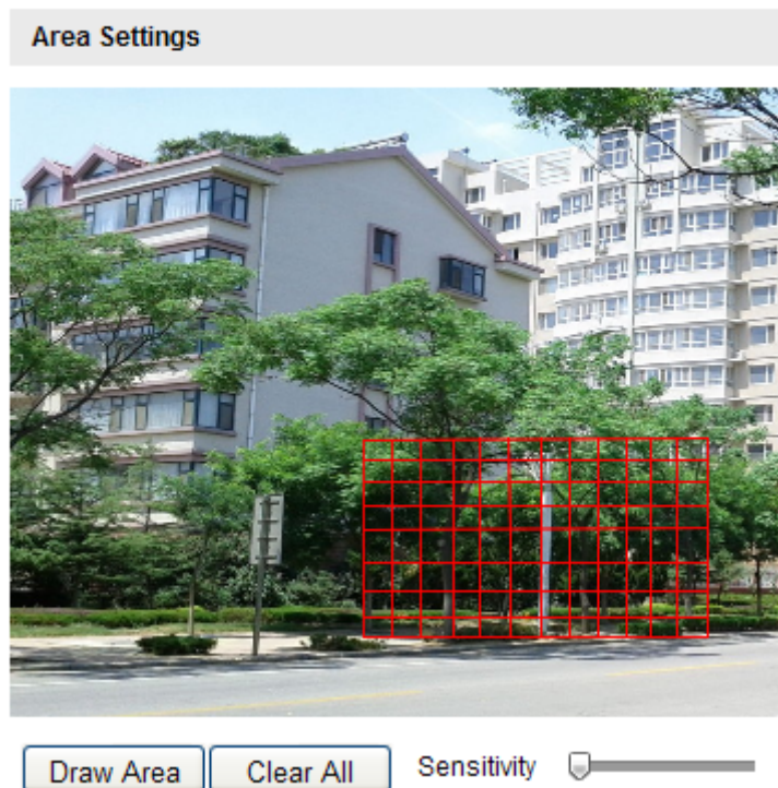
Figure 6-37 Enable Motion Detection
