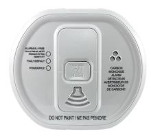
The ClareOne Carbon Monoxide Detector is a battery powered wireless detector that communicates with the ClareOne Panel. The detector consists of an electrochemical CO sensor and a wireless transmitter.
