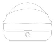
4.1.b Gently slide a fingernail/fingertip into the slot and push the top casing of the sensor upward.
