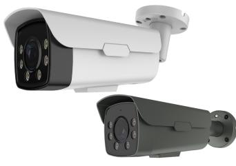
The 8MP ClareVision Bullet camera includes a Sony® Starvis™ image sensor with a 2.7-13.5 mm motorized varifocal lens that supports autofocus. The enables IR ngihtvision up to 60 meters, and supports smart detection capabilities such as human body detection, line crossing, loitering, intrusion, and people gather. The camera can be used standalone with an SD card or NVR, as well as accessed through a ClareOne or Control4 system.
