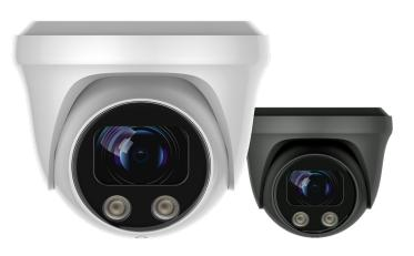
Featuring a 4MP, Sony® Starvis™ image sensor, this Performance Series ClareVision Turret camera includes a 2.8 mm lens with a maximum recording resolution of 2560 x 1440p at a stable 30 FPS. The camera includes support for True WDR and includes a 32 GB micro SD card for local, onboard storage.
