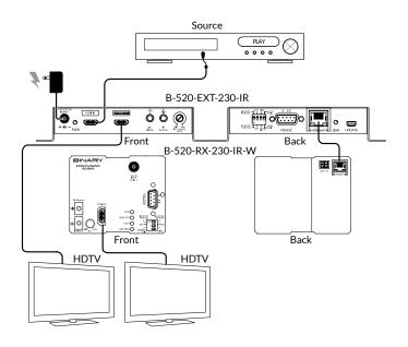
FIGURE 3: Application Diagram with non-PoC Transmitter
