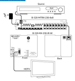
FIGURE 2: Application Diagram – Matrix Switcher
