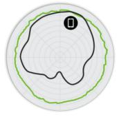
Figure 3. A750 5GHz AzimuthAntenna Patterns
