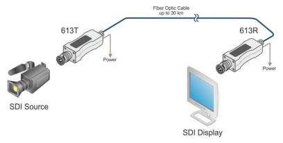
Figure 1: 613T, 613R 3G HD-SDI Mini Optical Transmitter/Receiver
