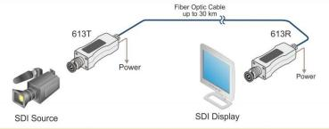
Always use Kramer high-performance cables for connecting AV equipment to the 613T/R.
