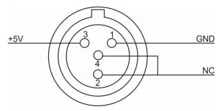
Figure 2: Power Connector Pinout
