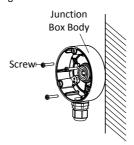
Figure 2-5 Fix the Camera to the Ceiling
