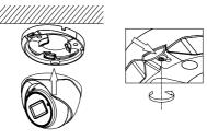
Figure 2-10 Install the Turret Camera
