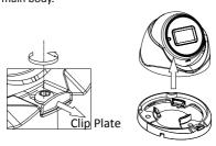
Figure 2-8 Remove the Clip Plate
