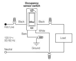
**Note**: When a neutral connection is available, remove the green sleeve and connect the white wire to neutral.
