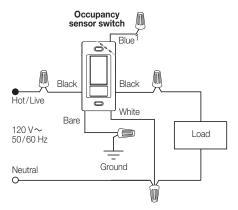
**Note**: When a neutral connection is available, remove the green sleeve and connect the white wire to neutral.
