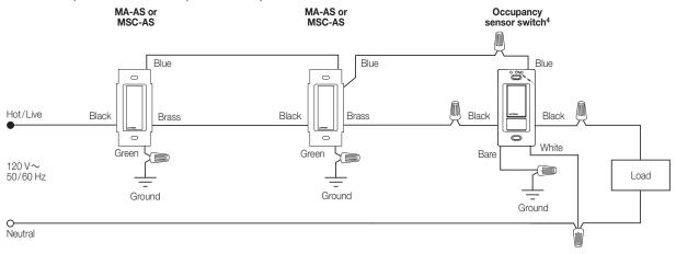
Note: When a neutral connection is available, remove the green sleeve and connect the white wire to neutral.
