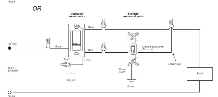
Note: Remove white sleeve and connect green wire to ground only in retrofit and replacement applications.
