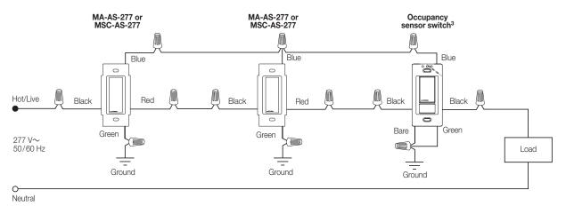
Note: Remove white sleeve and connect green wire to ground only in retrofit and replacement applications.
