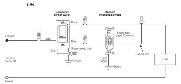
Note: Connect green-sleeved wire to ground only in retrofit and replacement applications.
