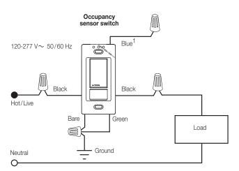
Note: Remove white sleeve and connect green wire to ground only in retrofit and replacement applications.
