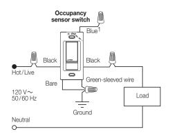
**Note**: Connect green-sleeved wire to ground only in retrofit and replacement applications.
