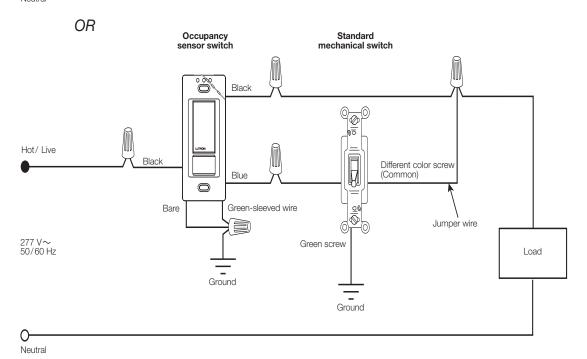
Note: Connect green-sleeved wire to ground only in retrofit and replacement applications.
