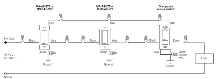
Note: Connect green-sleeved wire to ground only in retrofit and replacement applications.
