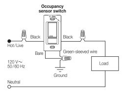
**Note**: Connect green-sleeved wire to ground only in retrofit and replacement applications.
