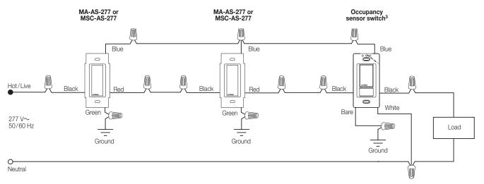
Note: When a neutral connection is available, remove the green sleeve and connect the white wire to neutral.
