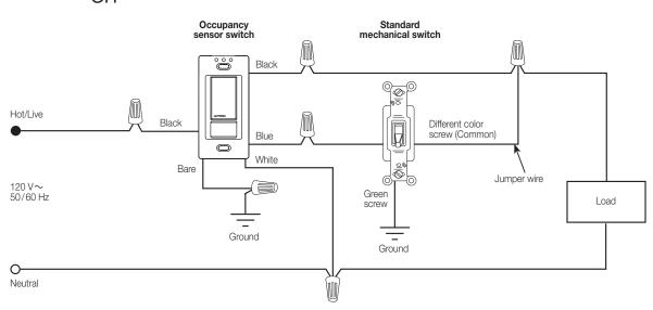
Note: When a neutral connection is available, remove the green sleeve and connect the white wire to neutral.
