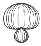
Mainly used in gooseneck microphones as only smaller volume adjustments are needed which allows greater freedom of movement towards/from microphone. In comparison to other microphones, super-cardioid mics allow for bigger distance between speaker and mic itself
