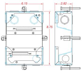
There are six ¾"-1" concentric knock-outs and four ¾" knockouts on the FL-200-3 box.
