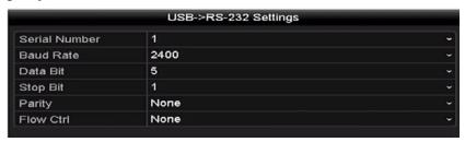
When using USB->RS-232 convertor mode, the port used on the USB-to-RS-232 convertor must match the POS number. For example, POS1 must connect to port 1 of the convertor.
